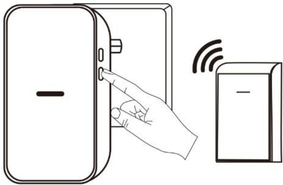
2 Clear code pairing: If the receiver is disconnected, press and hold the "volume control button", then turn on the power until you hear "bim bam, bim bam", then release your hand to clear all the code pairings in the device, then all the transmitters will disabled and will need to be re-paired.
